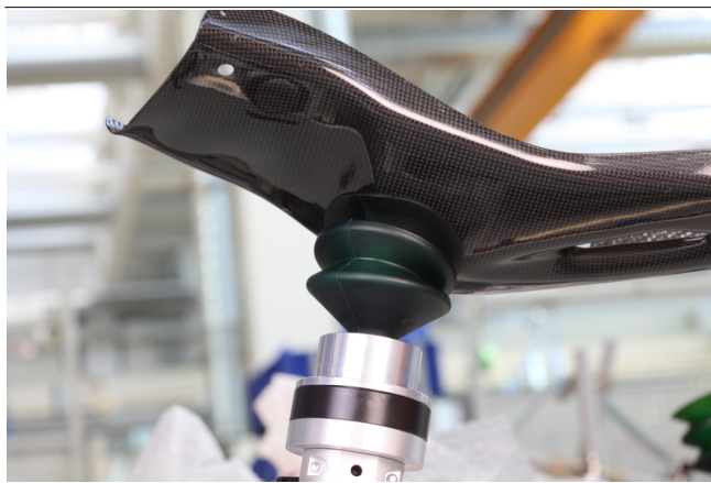
Uni-Base UB and reference suction cup RSC for clamping a CFRP part
