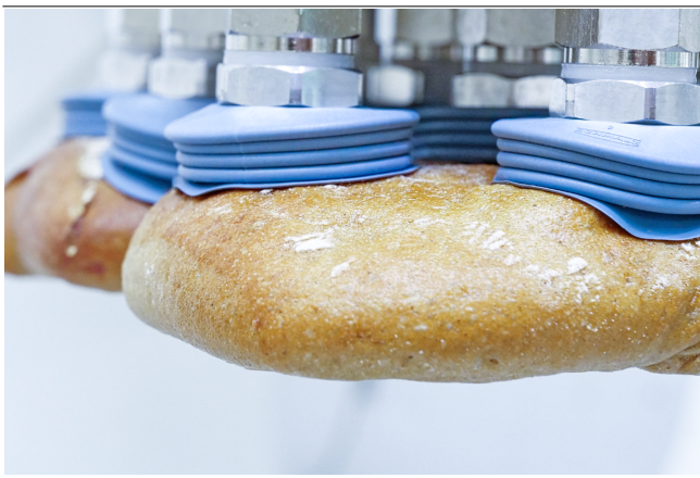
Bellows suction cups FSDC when handling baked goods
