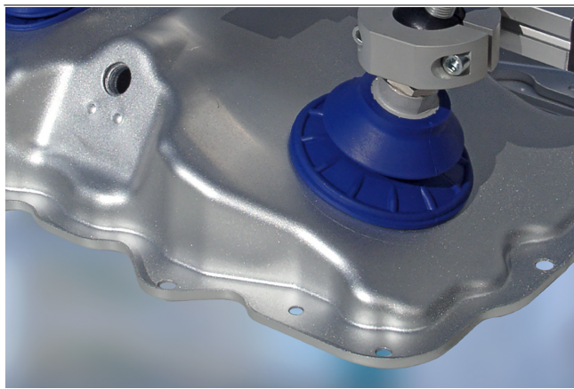
Bellows suction cups SAB being used for handling car bodywork parts
