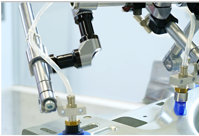
Cross beam connector (geared) SXT-TC in combination with holders HT-SG and suction cups SAX when handling an automotive part
