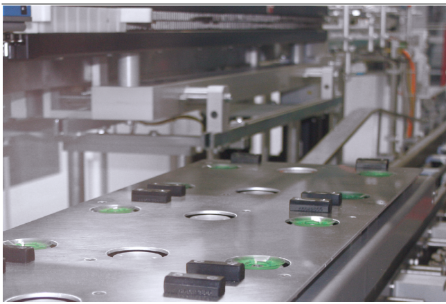
Flat suction cups SPF for use in carton erectors
