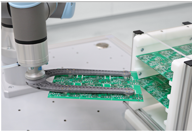
Floating suction cups SBS when handling printed circuit boards
