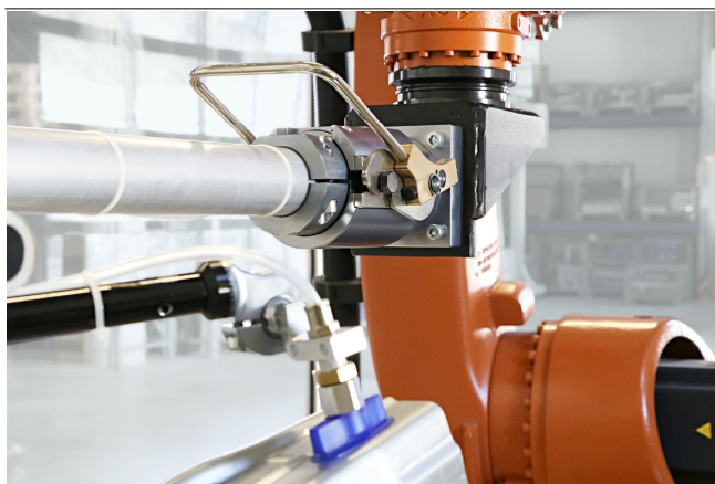
Quick-change robot bayonet SXT-QC-CON used for handling a formed sheet metal part
