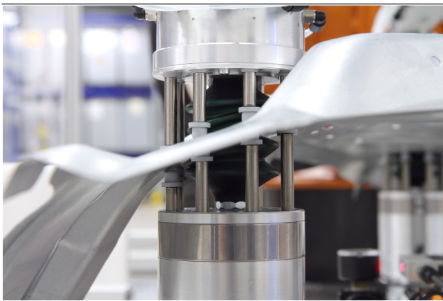
Suction Cup Balance SSCB for automated gripping and clamping of a sheet metal part
